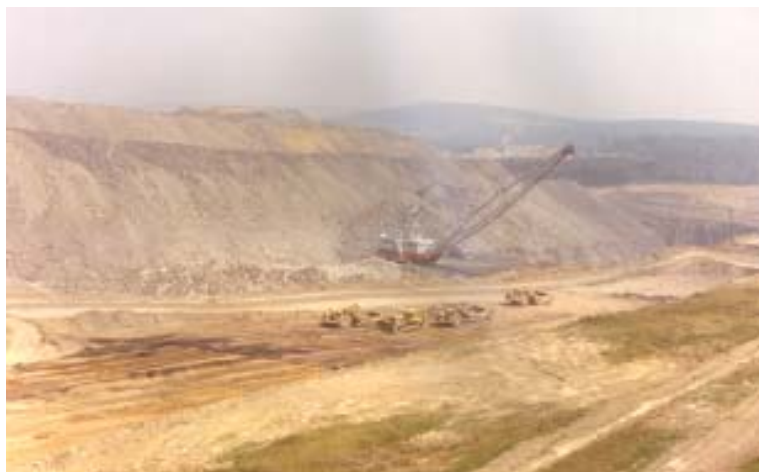
The extent of surface mining on the memorial property is evident in this photo from 1978-79. The large piece of red and white equipment is a dragline which removes soil and rock to expose seams of coal. ~ Photo courtesy of Marlin Sherbine
